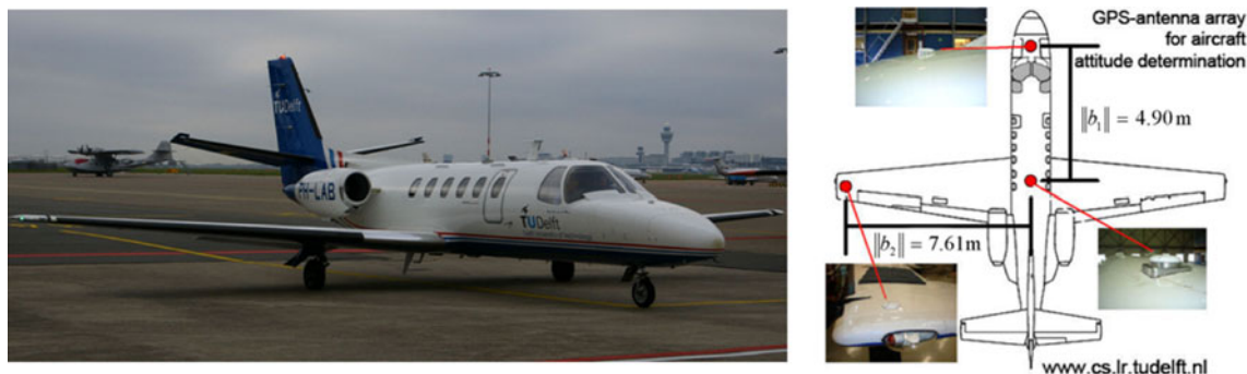
Fig. 7 The aircraft with antennae configuration
