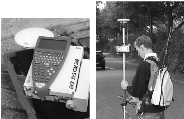
Figuur 9 Real-Time Kinematic (RTK) GPS surveying: the surveyor directly 'digitizes' the points of interest in the field, by holding the antenna accurately in place for just a few seconds.
