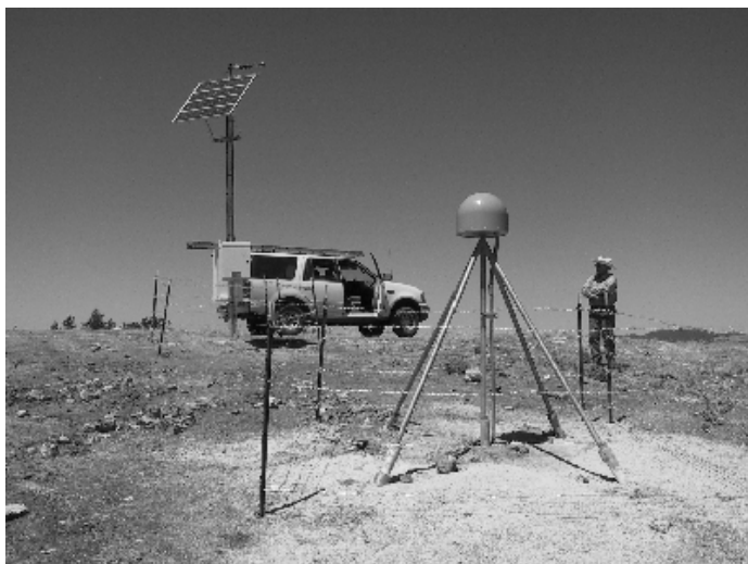
Figuur 2 A GPS receiver and antenna permanently installed for precisely monitoring motions of the earth's crust. Site Ranchita in California in the US. Photo taken from album at http://www.scign.org/
