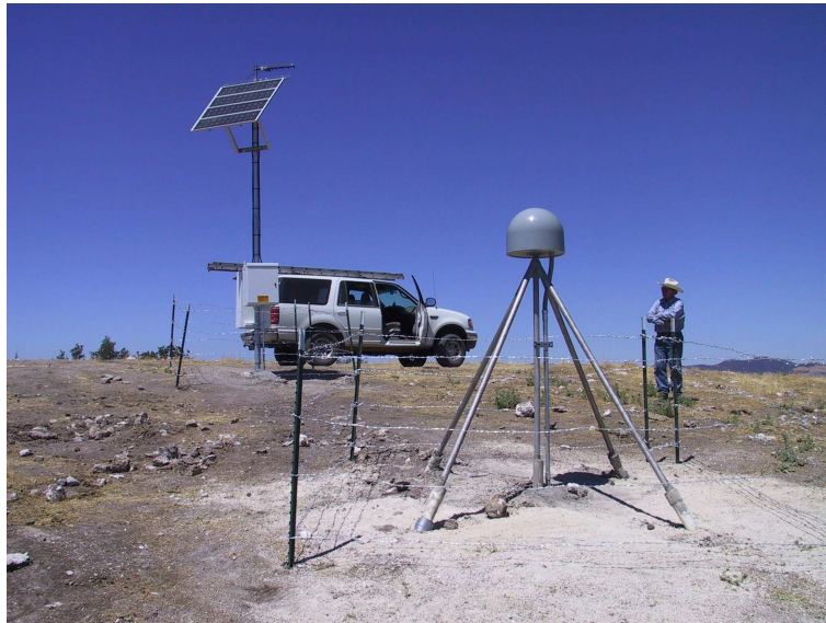
Figure 9: A GPS receiver and antenna permanently installed for precisely monitoring motions of the Earth's crust. Site Ranchita in California in the US. Photo taken from album at http://www.scign.org/
