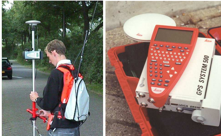
Figure 8: Real-Time Kinematic (RTK) GPS surveying: the surveyor directly 'digitizes' the points of interest in the field, by holding the antenna accurately in place for just a few seconds.
