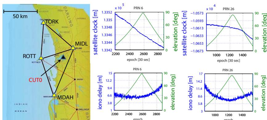
**Figure 1:** (Left) CORS network (yellow triangles) used for generating the PPP(-RTK) products for user location CUT0 (black triangle). (Right) Examples of ambiguity-fixed satellite clock and interpolated ionospheric delay estimates for full arcs of PRNs 6 and 26 during 23 October 2010, where an epoch interval is 30 sec is used. In the graphs the satellite’s elevation is plotted as well.
