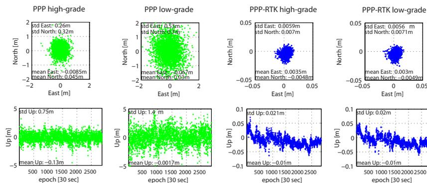
**Figure 3:** PPP and PPP-RTK positioning results based on single-frequency GPS phase and code data. It is remarked that the PPP results are obtained by epoch-by-epoch kinematic processing, while those for PPP-RTK are based on accumulation of epochs.
