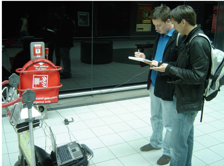
Figure 3. Luggage trolley with u-blox receiver connected to laptop, while patch antenna is held in hand.
