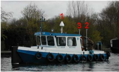
Figure 6. A picture of the ship used for the kinematic experiment. 1: choke-ring antenna connected to the Ashtech receiver 2: antenna connected to the Leica SR530 receiver 3: antenna connected to the Novatel OEM3 receiver
