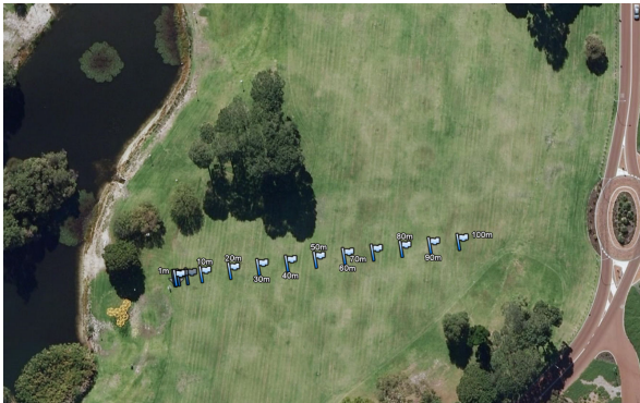
Fig. 1. Placement of the receivers on field
