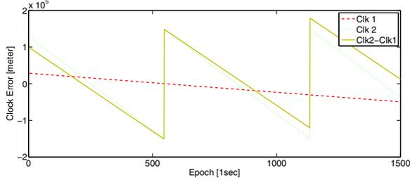
Fig. 3. Clock errors and the difference for the two GPS receivers
