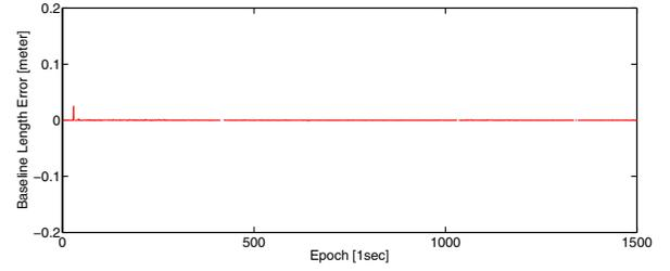
Fig. 7. Baseline error using the proposed double difference model for both receivers
