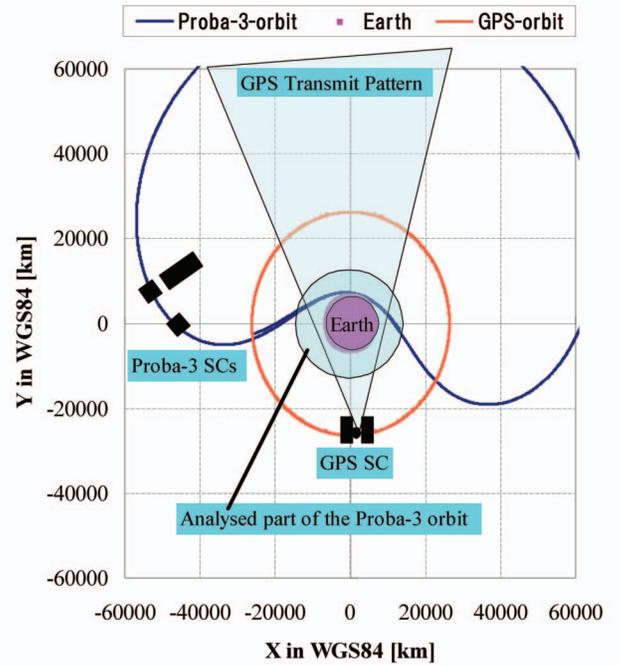
Fig. 1. Orbits of Proba-3 and GPS spacecraft (SC)
