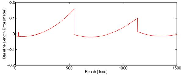
Fig. 4. Baseline error using the standard double difference model
