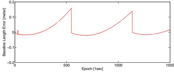
Fig. 5. Baseline error using the proposed double difference model only for receiver 1
