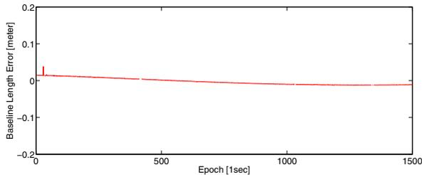
Fig. 6. Baseline error using the proposed double difference model only for receiver 2
