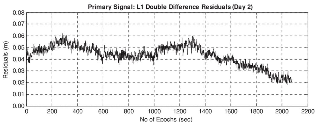
Figure 1. Double difference residual time series for satellite pair 16-20
