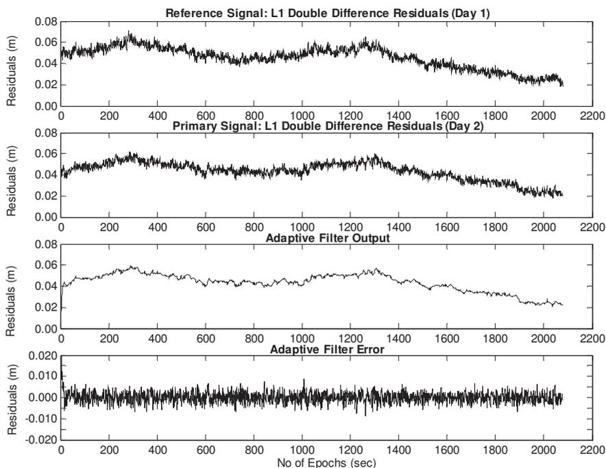
Figure 6. Adaptive filter applied to L1 double-difference residuals of satellite pair 16-20
