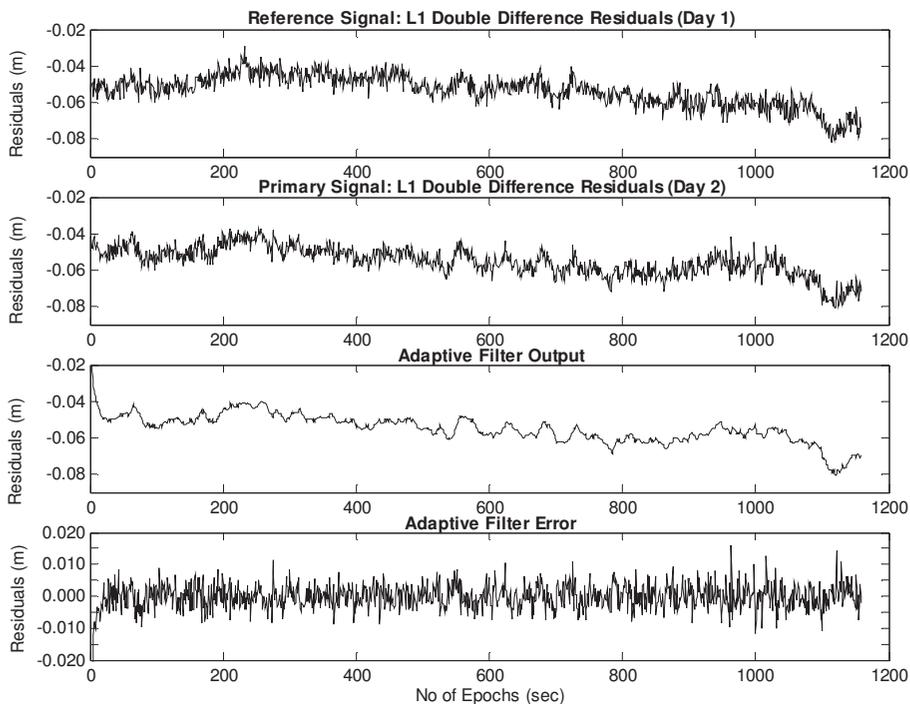
Figure 7. Adaptive filter applied to L1 double-difference residuals of satellite pair 20-1
