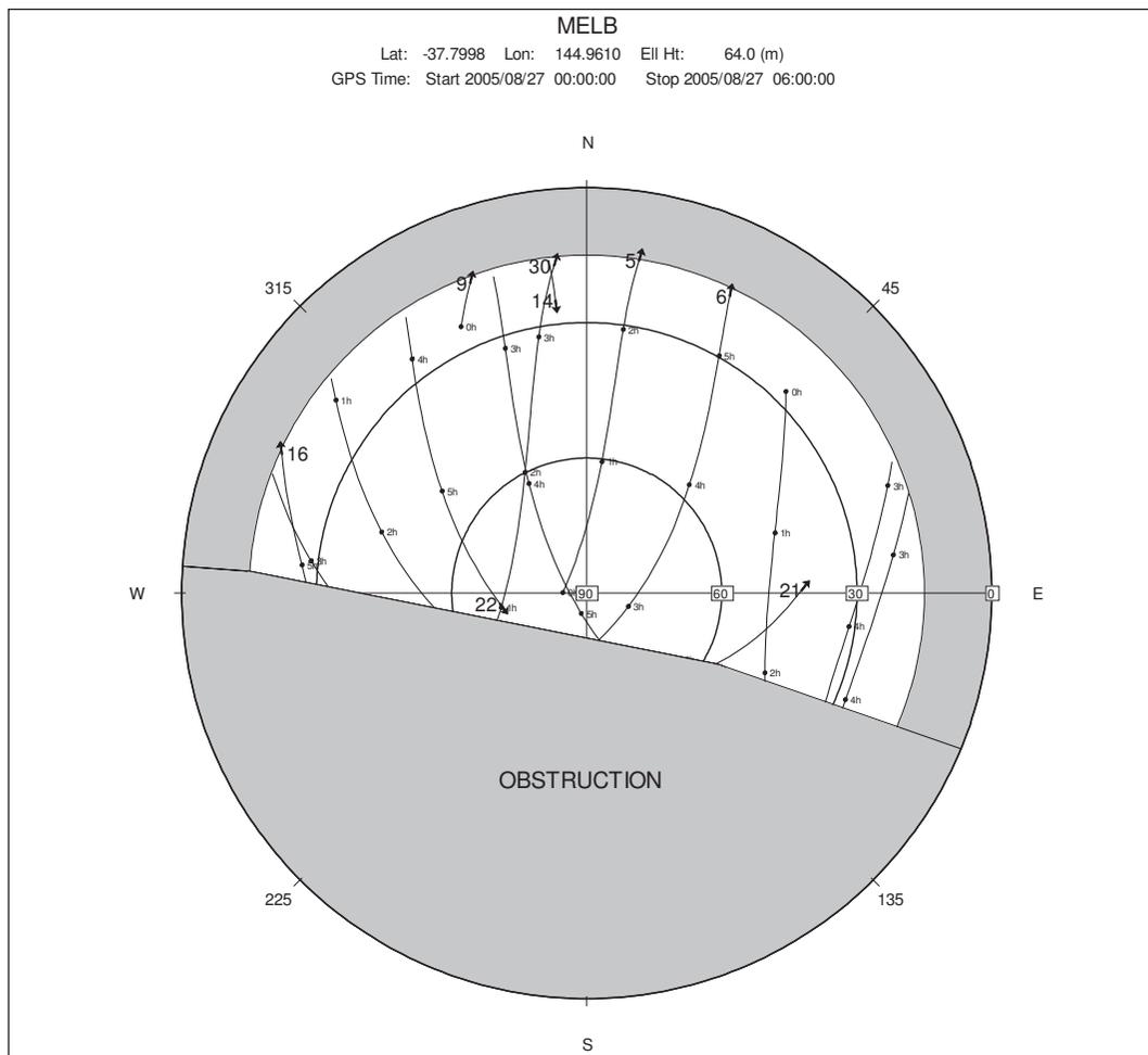
**Figure 5.** Obstruction map of the receiver site (created using *skyplot.exe*, Marshall 2002).
