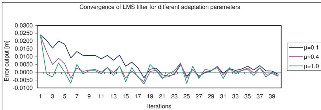
**Figure 3.** Convergence rates for satellites 16-20 using different adaptation parameters
