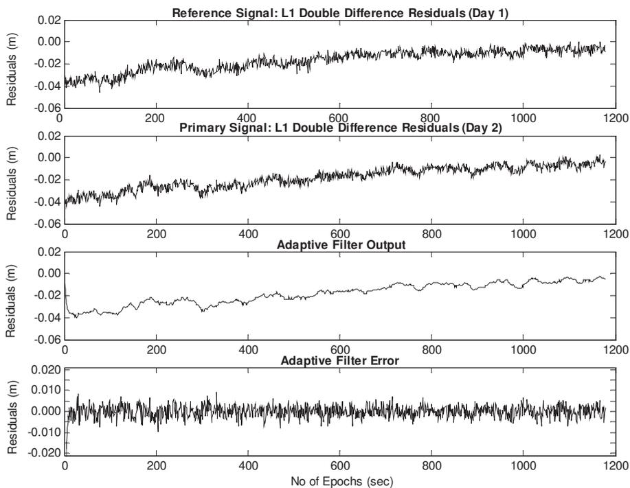
Figure 8. Adaptive filter applied to L1 double-difference residuals of satellite pair 20-24
