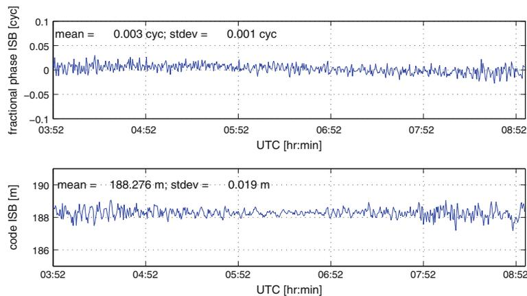
**Fig. 11** Estimated differential L5–E5a ISBs for phase (*top*) and code (*bottom*) for USN4–USN5 (04/03/12), a Novatel and Septentrio receiver in a zero-baseline setup, based on GPS and GIOVE-A data
