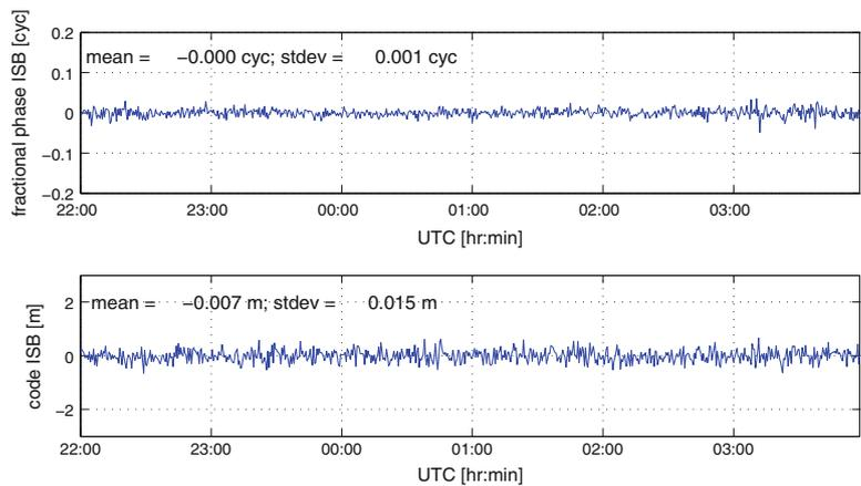
**Fig. 7** Estimated differential L5–E5a ISBs for phase (*top*) and code (*bottom*) for CUT0–CUT1 (21–22/05/11), a Trimble and Septentrio receiver in a zero-baseline setup, based on GPS G25 and GIOVE-B data
