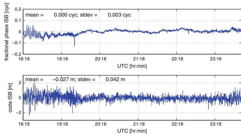
**Fig. 2** Estimated differential L1–E1 ISBs for phase (*top*) and code (*bottom*) for the Muresk experiment (08/06/11), for Javad and Trimble receivers, separated by 0.5 m, based on GPS and GIOVE-A data
