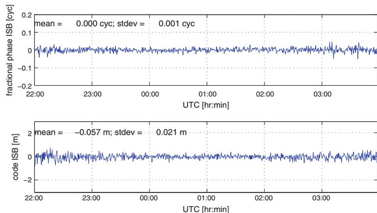
**Fig. 5** Estimated differential L1–E1 ISBs for phase (*top*) and code (*bottom*) for CUT0–CUT1 (21–22/05/11), a Trimble and Septentrio receiver in a zero-baseline setup, based on GPS and GIOVE-B data
