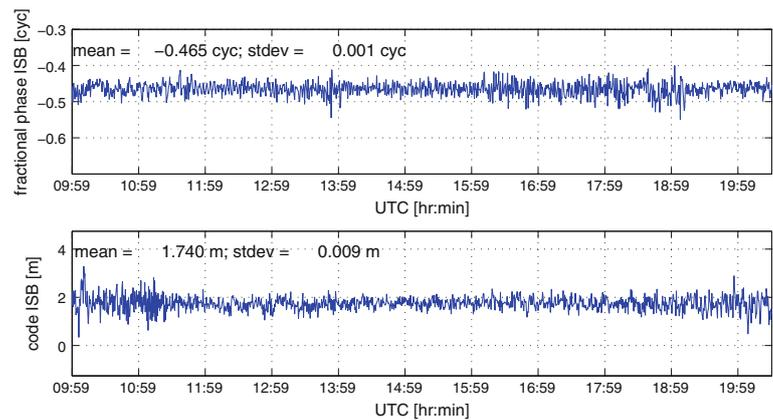
**Fig. 9** Estimated differential L1–E1 ISB results for 07/11/11: CUT1–CUT3 (Septentrio–Javad). The time series start later than in Fig. 8, since CUT1 was only able to track GIOVE-A much later than CUT3 (only at the time GIOVE-B was observed as well)
