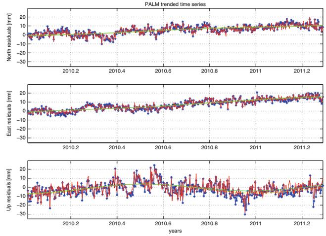
**Fig. 4** Example of a time series showing secular and periodic motion (PALM station), GPS (blue line), GPS + GLONASS (red line), green solid line is the fitted model
