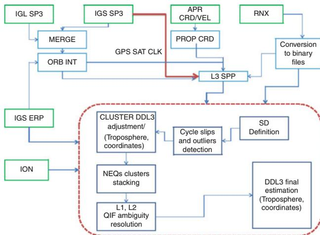
**Fig. 2** Processing strategy used for the combined GPS + GLONASS processing: *green boxes* represent the input information, *light blue boxes* point out the main steps of the pre-processing, *dark blue boxes* enclosed by the *dashed line* represent the double difference processing, *blue lines* describe the processing flow
