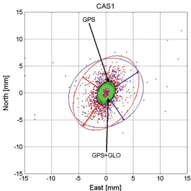
**Fig. 6** CAS1 scatterplot derived by SINEX files, *black and green ellipse* (95 %) computed on the basis of the formal VCV matrix
