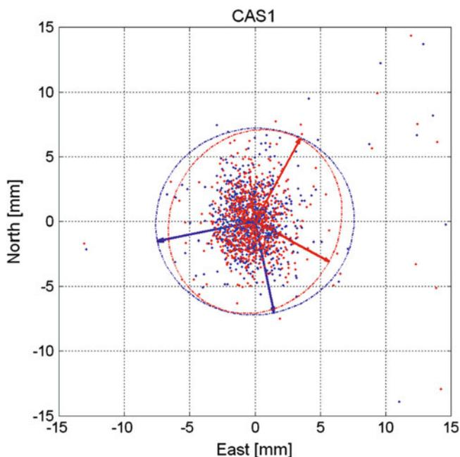
**Fig. 7** CAS1 scatterplot derived by CATREF residuals. The reference frame effects have been absorbed by the reference frame parameters, therefore the error ellipses (95 %) are less elongated than their counterparts in Fig. 6
