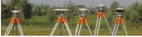
Figure 2. Arrays of five antennas used in the experiment setup at Delft University of Technology (20 m baseline)
