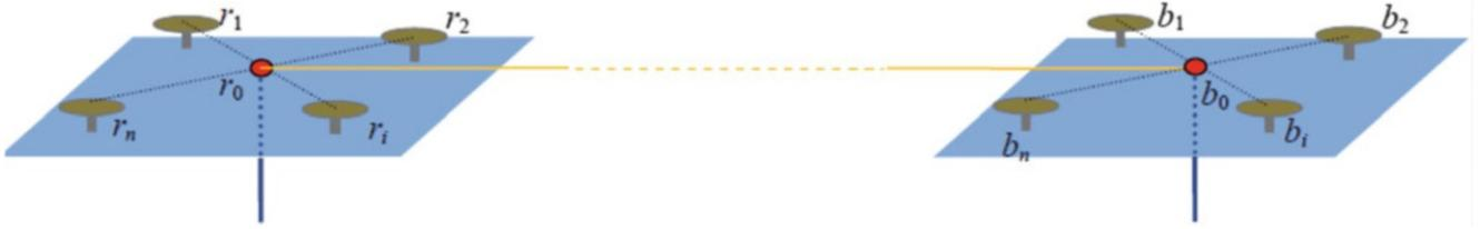
**Fig. 1** The layout of antenna-array at two platforms,  $r_0$  and  $b_0$ , of one baseline. An array of antennas,  $r_1, r_2, \dots, r_n$ , are mounted on the platform  $r_0$ , and the antennas,  $b_1, b_2, \dots, b_n$  on the platform  $b_0$
