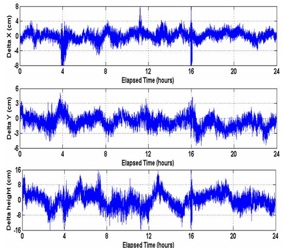
Fig.14. Positioning series based on ionosphere-free combinations of DD L1 and L5 phases
