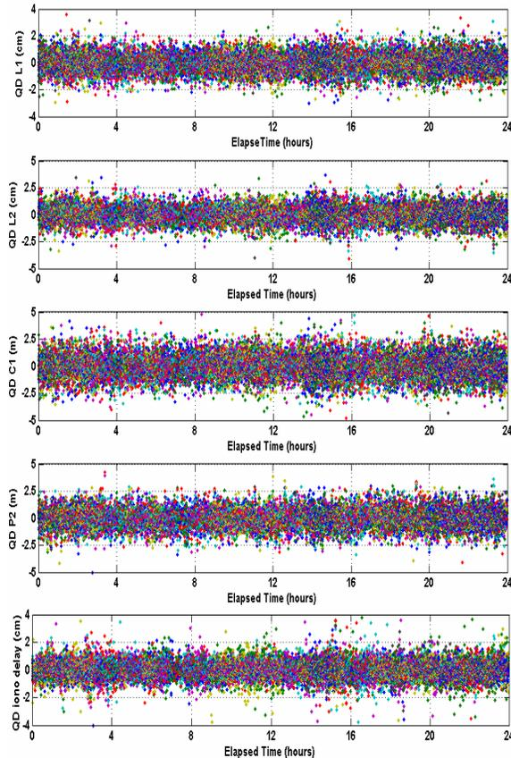
Fig.6. QD observation series respectively for L1, L2, C1, P2 and ionospheric delay
