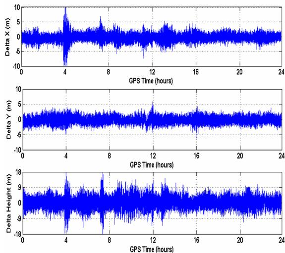
Fig.16. Positioning series based on ionosphere-free combinations of DD P5 and C1 codes
