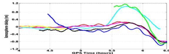
Fig.3. Variation of DD ionospheric delay for some pairs of DD satellites in the ionosphere disturbance period
