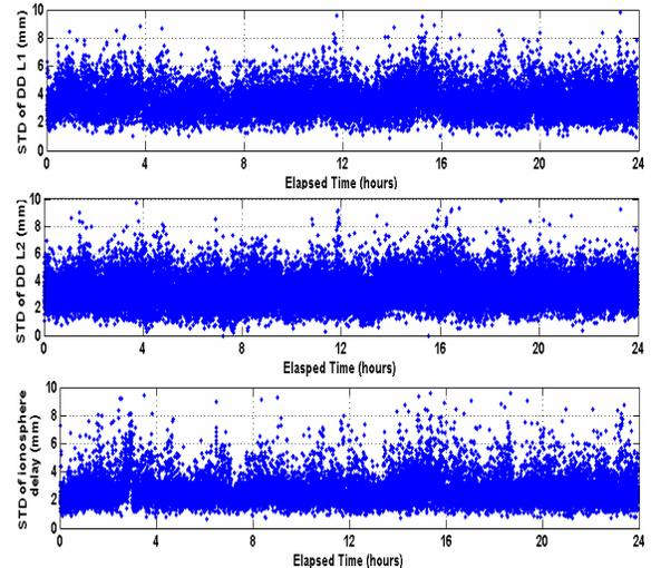
Fig.7. STD series of DD L1, DD L2 and DD ionospheric delay
