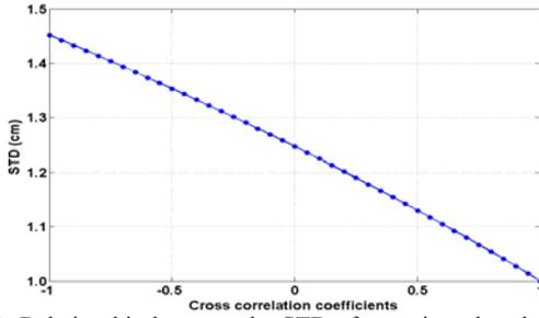
Fig.1. Relationship between the STD of error introduced at DD L5 and the cross correlation coefficients between L1 and L2 phases
