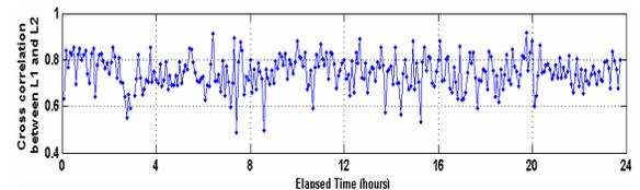
Fig.9. Cross correlation coefficients between L1 and L2 phases
