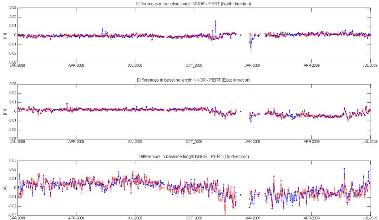
Figure 2: North, East and Up baseline length differences NNOR-PERT compared to the mean baseline length for the complete network (red) and the small network (blue).
