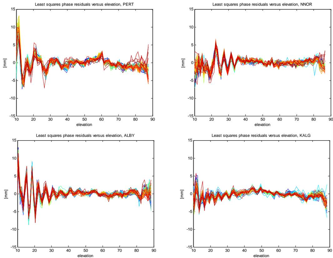
Figure 8: Undifferenced least squares phase residuals per elevation for selected stations for 61 days, each day has a different colour.
