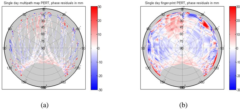
Figure 3: Single day multipath map (a) and finger-print (b) for PERT. The multipath map shows the stacked residuals, the finger-print is an interpolation of the multipath map.
