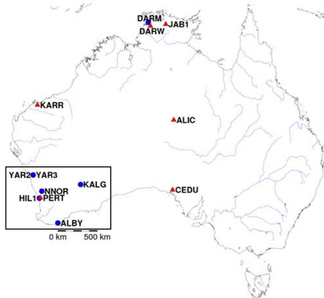
Figure 1: Selected CORS network to obtain undifferenced residuals, stations inside the black rectangle form a smaller sub network. Red triangles indicate IGS reference frame sites.
